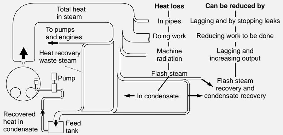
Figure 3: Where the heat goes and what can be done to reduce losses [15].
