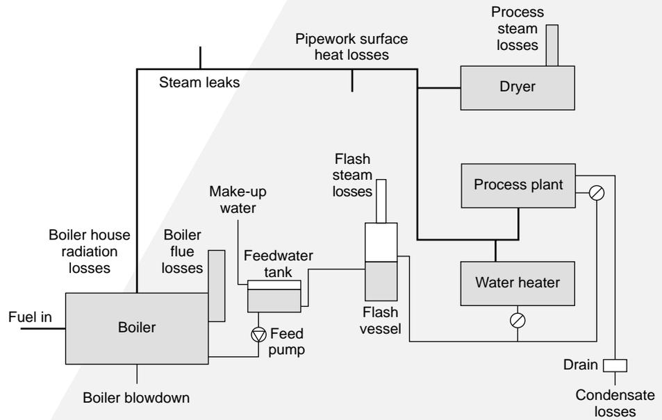
Figure 2: A simple steam system showing main areas for improving energy efficiency.
