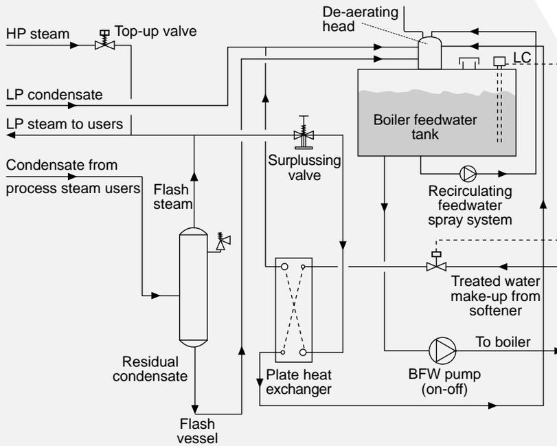
Figure 5: Flash steam recovery system and feedwater tank.
