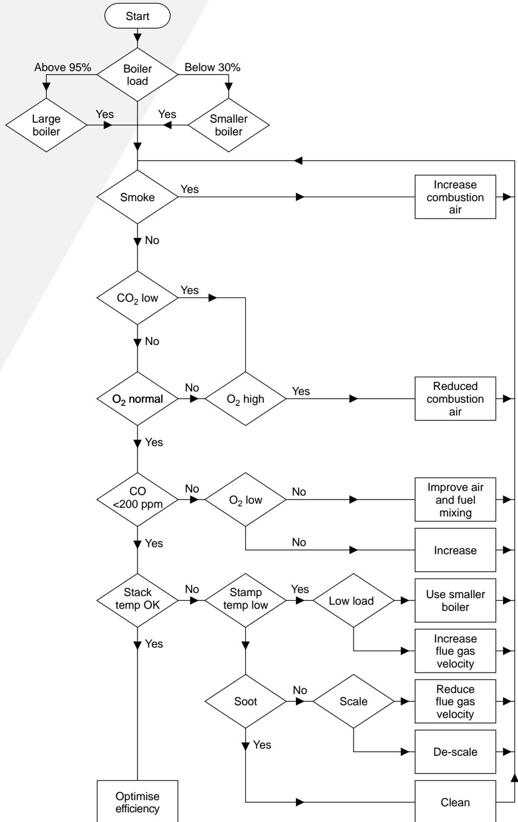
Figure 4: Flow diagram of efficient boiler operation [1].
