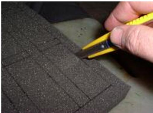
This is where you need the really sharp knife. A sharp one will quickly and easily slice through the foam requiring little sawing action. This may take a little practice, but about 5 minutes you will have the idea! Keep the knife as upright as you can, and cut about 90% of the way through both the long and short areas of it. The reason for not cutting right through will be shown in the next steps.
