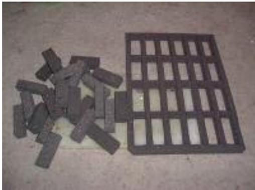
Finish the cutting of the pieces. I found that if you bend the foam slightly, it is easier to see the cut-outs and also see where it is still joined. Try not to over cut into the main block of foam. You only require the cut-out areas to be sliced out!
