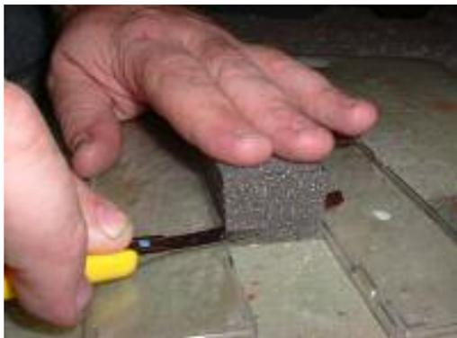
Next you have to cut the bases for the holes. Use something hard that is 5mm thick as a base. The picture shows 2 Life Like train tops from their plastic packaging. These are 5mm thick, and perfect for the job. By bending the blade slightly, you can get a straight cut of 5mm by a slight sawing action across the two tops as shown in the photo. Once again, a sharp blade does a terrific job! Ensure that the numbered side is facing down!
