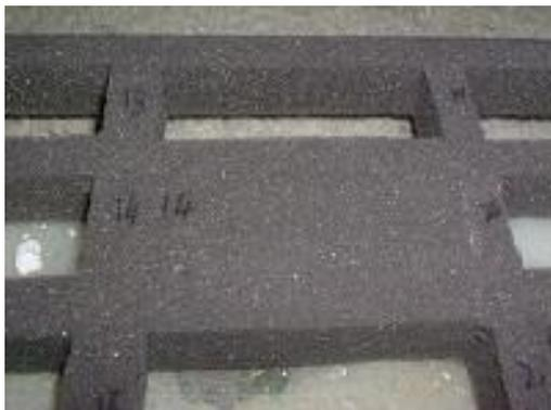
Use the Tarzans Grip and glue the 4 sides of the base piece to put in. As in the picture, put in place by slightly opening the cut-out areas and place the section in while the whole lot is upside down. Turn the whole thing the correct side up on a flat surface and push down lightly on the piece you just glued in making it level with the bottom of the main piece. Turn it upside down again and check it is level. Ensure all corresponding numbers are correct!
