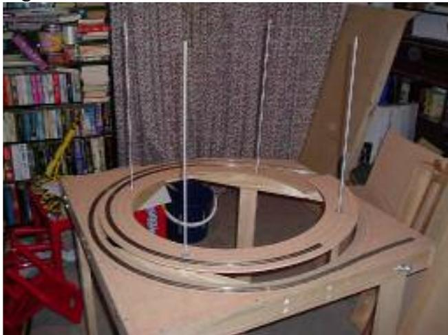
Once most of the track work for the first layer is in place, then put the uprights in. These should slot neatly and tightly into the slots you drilled earlier. To make the levels lock into place, then put one nut and washer on the bottom and another on the top. When you tighten the nuts up in a minute, then they will lock the wood in place.
