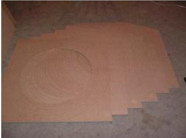
Here are the next sections for the helix already cut. There are 6 sections here, making 7 sections all up. The finished elevation will be 48cm above the point where it started off.
