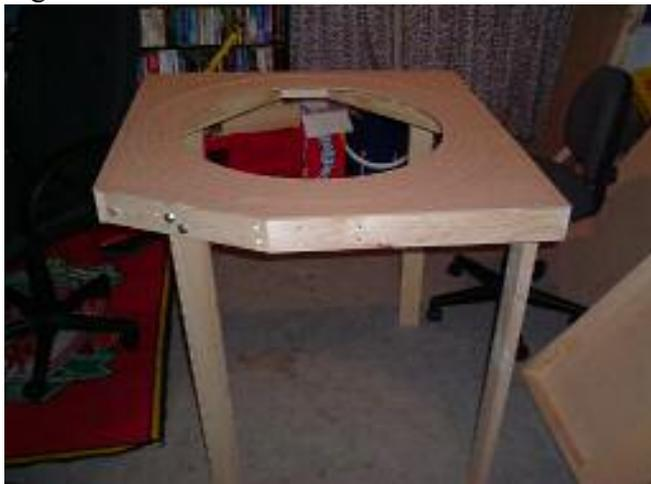
Before you cut the wood for the helix so you can get inside in case of accidents, mark the middle of the board, drive a nail in the center and then draw circles from the edge coming in. This will be the guide lines for the track, as the track here will not have any underlay on it. I had a straight bottom layer and the helix started on the inside. Cut the wood for the rise before you go to the next step.
