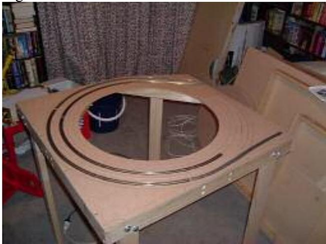
Lay the first row of tracks. I have a loop on the bottom and the helix on the inside. As the trackage gets to the next level, it will move out one drawn ring. Determine where the tracks are going to enter the board and exit. I used a program called XTrackCad as it can print to a scale of 1 to 1 so you can print the sections and place them onto your work to get the track work right.
