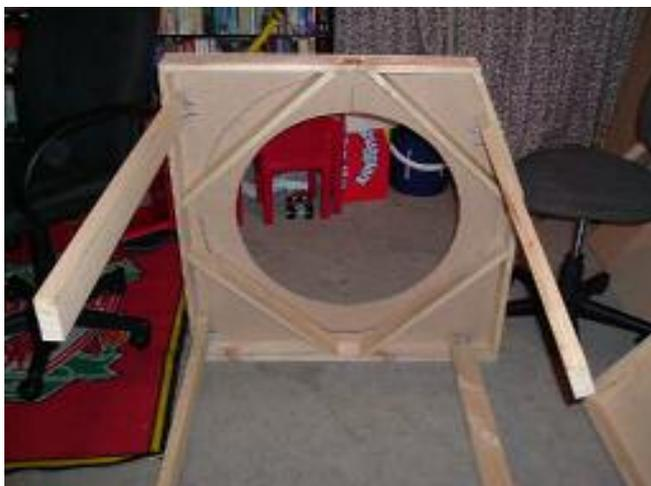
I made the inside cut-out 62cm. This is a good size for an average sized person to get up inside of. I then made 4x 45 degree supports. I did this so that the supports will take the pressure of the uprights and the other layers (Fig 2) without depending on the strength of the bottom layer alone. Drill the holes through the top and halfway into the supporting wood for the uprights to sit neatly and tidy in. (see Fig 5)
