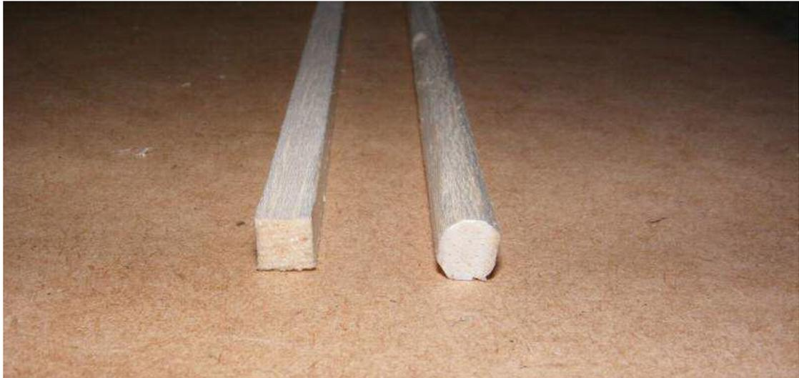
Cut the Balsa sheet so it is a square of 6.5mm x 6.5mm as the left of the picture show. Trim a small amount off the edges to make it into an octagon shape (8 sides) similar to the right hand picture.
