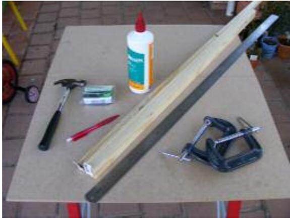
Here are some of the basic tools I use. Hammer, nails, glue, 6mm MDF, sharp pencil, a 1m metal ruler and G clamps.
