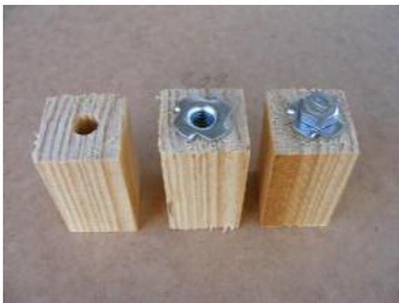
Drill a 3/8" (8mm) hole through the center of the 30mm x 30mm wood. Using 5/16" (M6) Tee Nuts, hammer them carefully into the wood. If you hammer them in gently where the spikes are, they go in nicely. Be careful not to split the wood when you hammer them in. Sometimes this can not be helped, and you can still use them anyway. Screw the bolt (all threaded) into the Tee Nut and your adjustable legs are ready.
