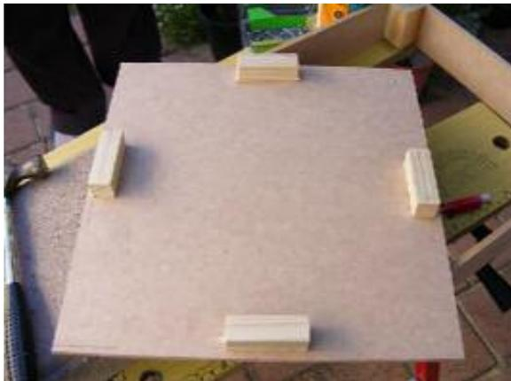
Here you see the top with the strengtheners on. I used a spare piece of 6mm MDF to space them out in the correct dimensions. I nailed and glued these so they will support the top to the sides as extra strength. Glue all connecting edges and put the top onto the box with adjustable legs. Nail and/or clamp them until dry.
