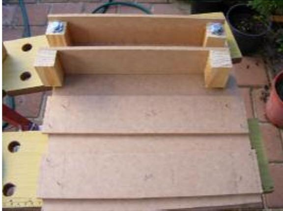
Once the legs are ready, you can attach them to one of the side panels. Use the shorter panels and it is easy to line them up with the edges of the legs. This means that you can put the front and back panels flush to the sides of the legs and side panels. Glue the two pieces together and nail them so they are secure.
